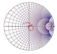
Figure 2. Input impedance varying the input power from -15 dBm to 10 dBm.
