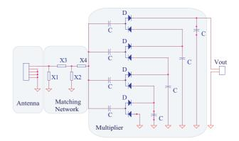
Figure 1. Schematic of the RF design
