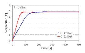
Figure 5. Charge of  $4700 \,\mu F$  and  $2200 \,\mu F$  energy buffer with  $5 \, dBm$  of input power at antenna.
