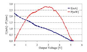
Figure 3. Characteristic of the harvester with 5 dBm of input power
